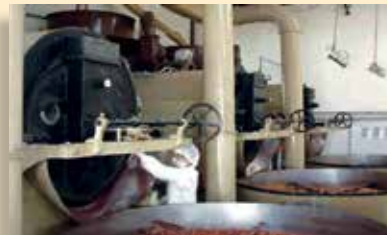
Lilla roasters, model T, manufactured in the 50's presently working at Inam's plant in Sao Paulo
